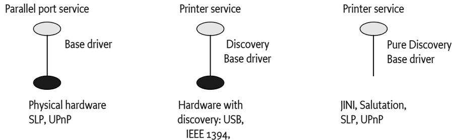
Base drivers discover physical devices using code not specified here (for example, through notifications from a device driver in native code) and then register corresponding Device services.
