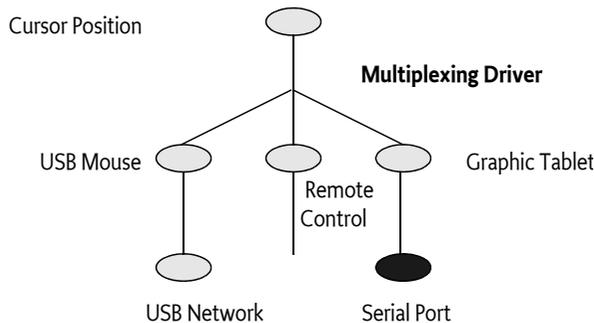
For example, assume that a system has a mouse on USB, a graphic tablet on a serial port, and a remote control facility. Each of these would be registered as a service with the Framework. A multiplexing driver can attach all three, and can merge the different positions in a central Cursor Position service.
