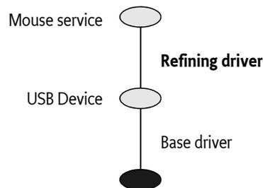
An example of a refining driver is a mouse driver, which is attached to the generic USB Device service representing a physical mouse. It then registers a new Device service which represents it as a Mouse service, defined elsewhere.
