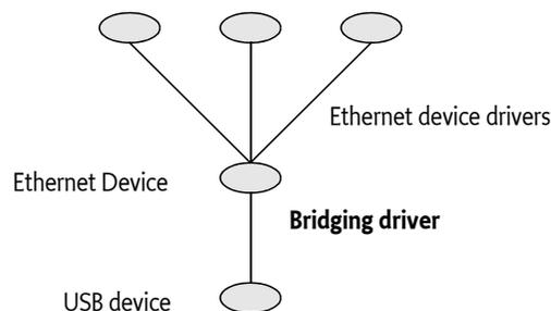
For example, USB to Ethernet bridges exist that allow connection to an Ethernet network through a USB device. In this case, the top level of the USB part of the Device service stack would be an Ethernet Device service. But the same Ethernet Device service can also be the bottom layer of an Ethernet layer of the Device service stack. A few layers up, a bridge could connect into yet another network.
