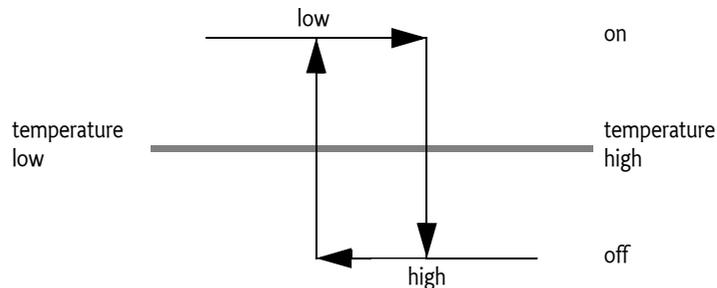
A Consumer service that controls the heater is only interested in events at the top and bottom of the hysteresis. If the specified high value is 250 °K and the specified low value is 249 °K, the following filter illustrates this concept:
